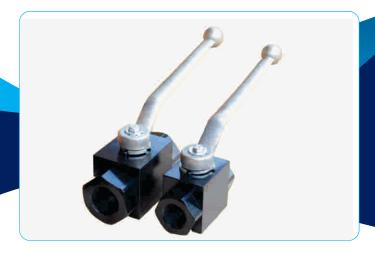
Lines operating under high pressure, typically around 300 bar, require high pressure ball valves for ON/OFF application. These valves are specially designed to withstand continuous use under these severe conditions. The Material of Construction is **MS** & **Stainless Steel**. These type valves can be supplied in round and square body.
